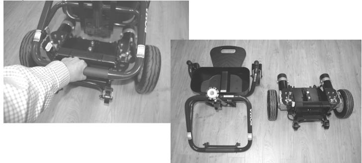
To reassemble locate the pivot pin of the front chassis into the receiving slots of the rear chassis (each side) and lowered to the bottom location.
