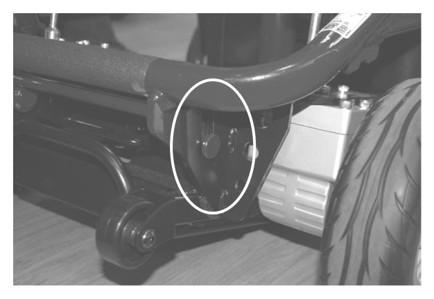
Push down on the rear part of the frame as shown below. This will reconnect the two parts of the frame together. You will hear the latch 'click' into place.
