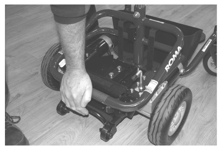
Refit the battery box and seat and reconnect the joystick. The scooter is now ready for use.
